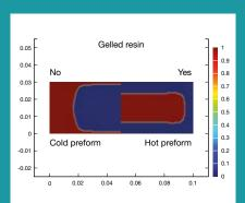
Optimize your part with the right preform heating strategy, e.g. to steer the gelation profile to be able to apply pressure during cure.
